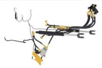
• Steering system uses a dedicated pump with dual double acting cylinders.
